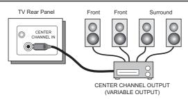
1) Connect the Pin cable from the TV's CENTER CHANNEL INPUT terminal to the surround amplifier's CENTER CHANNEL OUTPUT terminal.
